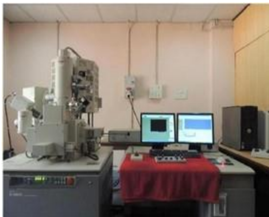
Figure 3.6: Field Emission Scanning Electron Microscope (FESEM) (Hitachi S-4800).
