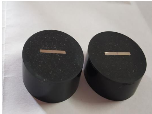
Figure 4.3 Mounted samples for microstructural inspection after welding
