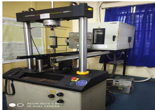
Figure 4.4 Experimental set up of INSTRON- 8801 for tensile test
