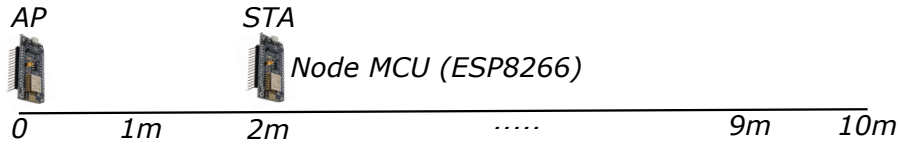
Figure 4.1: Distance estimation strategy in a straight line between AP and STA.
