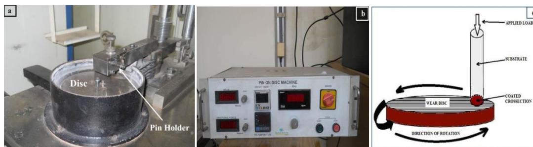
Figure 4.2 Comprehensive outline of Pin on Disc Machine (a) Pin on disc set up, (b) Data acquisition system, (c) Model showing rotational direction of disc
