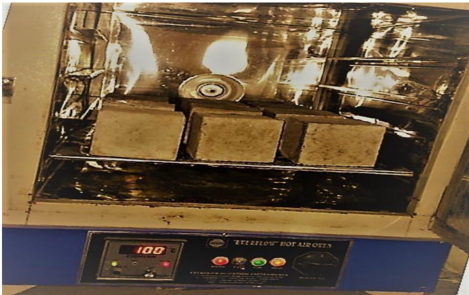
Figure 6 : Thermal resistance test of geopolymer mortar samples
