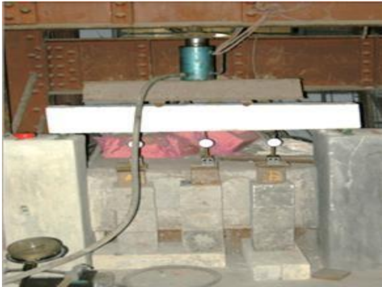
Figure 4 : Flexural strength test setup for reinforced concrete beam.
