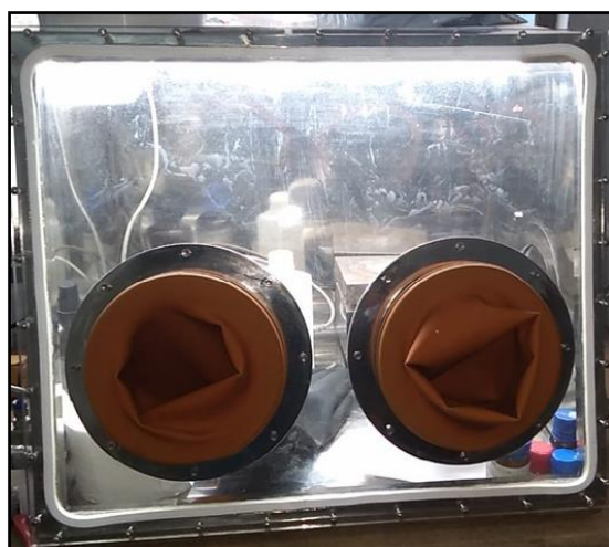
Figure 3.7: Shows self-designed laboratory glove box setup for Sn-based perovskite synthesis
