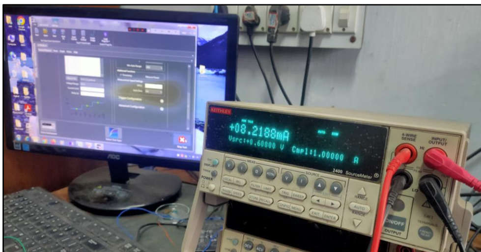
Figure 3.6: Keithley 2400 SMU with computer interface for the electrical measurements
