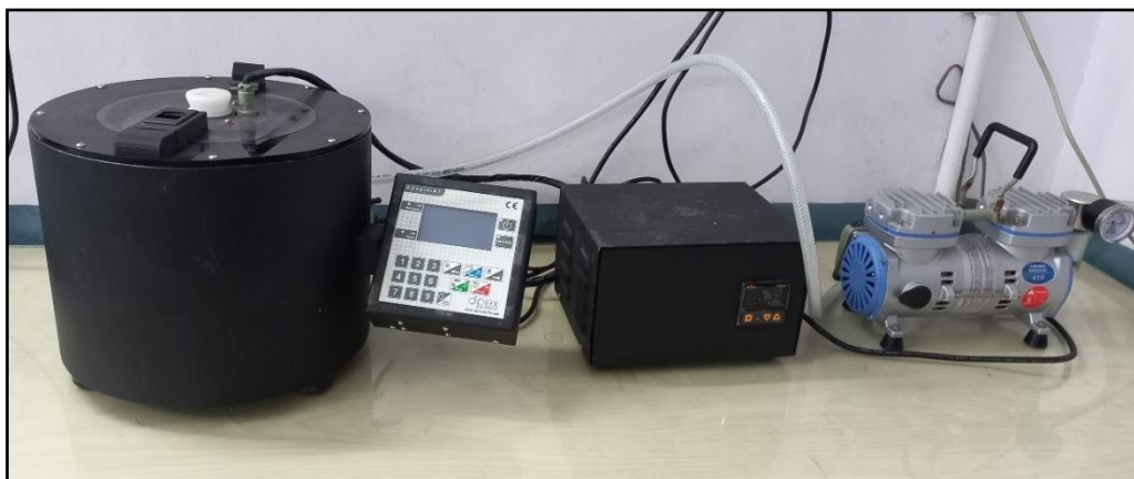
Figure 3.1: Spin coating setup for development of thin film.
