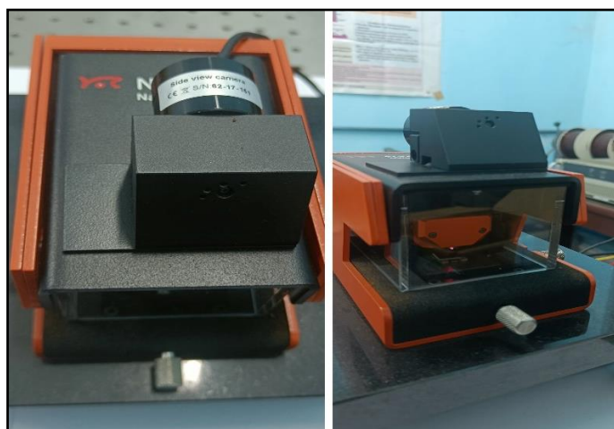
Figure 3.5: Shows laboratory AFM setup to measure film roughness
