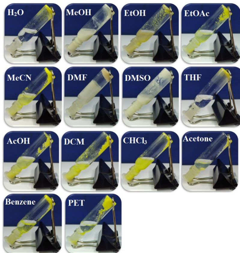
Fig. 3.3: Role of versatile solvents in forming stable metallogel of Mn-ATA.
