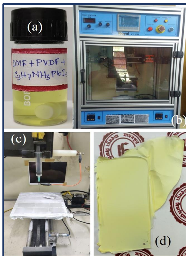
Fig. 3.2. a) The solution of C_3H_7NH_3PbI_3 +PVDF+DMF, b) Electrospin set-up, c) PVDF nanofiber formation, d) 4.76 wt% of C_3H_7NH_3PbI_3 incorporated PVDF nanofiber.
