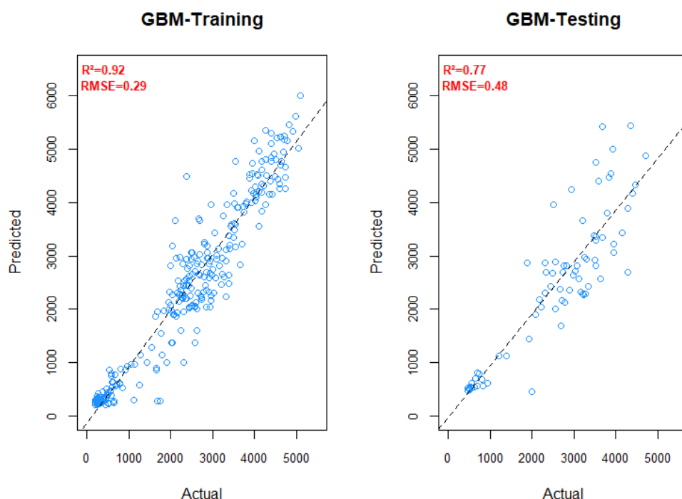
Fig. 10.6 Scatter plot between Predicted and Actual ^{222}\text{Rn} Concentration during training and testing period for (a) PCR (b) SVR (c) RF and (d) GBM. R^2 and RMSE values have been mentioned in the top of the plot in red.
