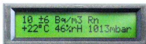
Fig. 4.4 Display showing radon concentration and other parameters
