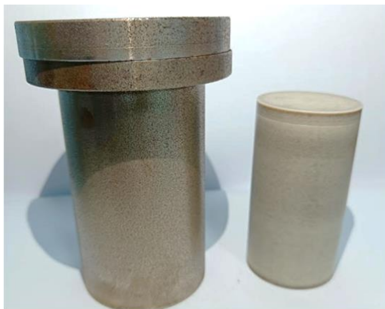
Fig. 2.1. Teflon chamber and stainless-steel chamber where all the synthesis were carried out.
