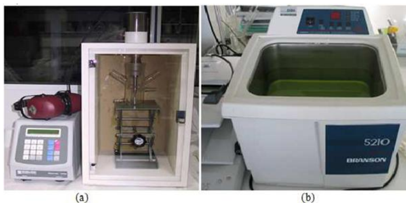
Fig.1.7: Common Type Ultrasound-assisted Extraction Unit: (a) Ultrasound Probe, (b) Ultrasound Bath (Source: Chemat, 2011)
