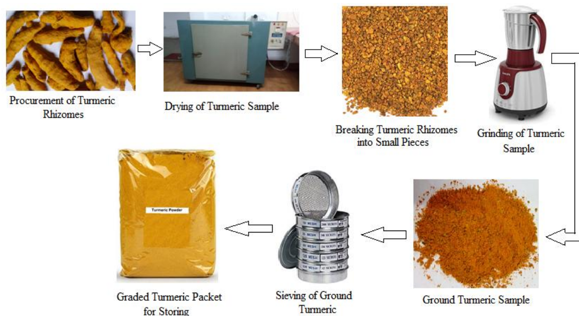
Fig. 5.2: Preprocessing Steps of Turmeric Rhizomes before SCO 2 E
