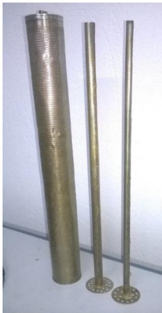
Fig. 4.4: Concentric Channels of 0.75cm and 1.5cm Diameters and 5.5cm Diameter Cylindrical Shell
