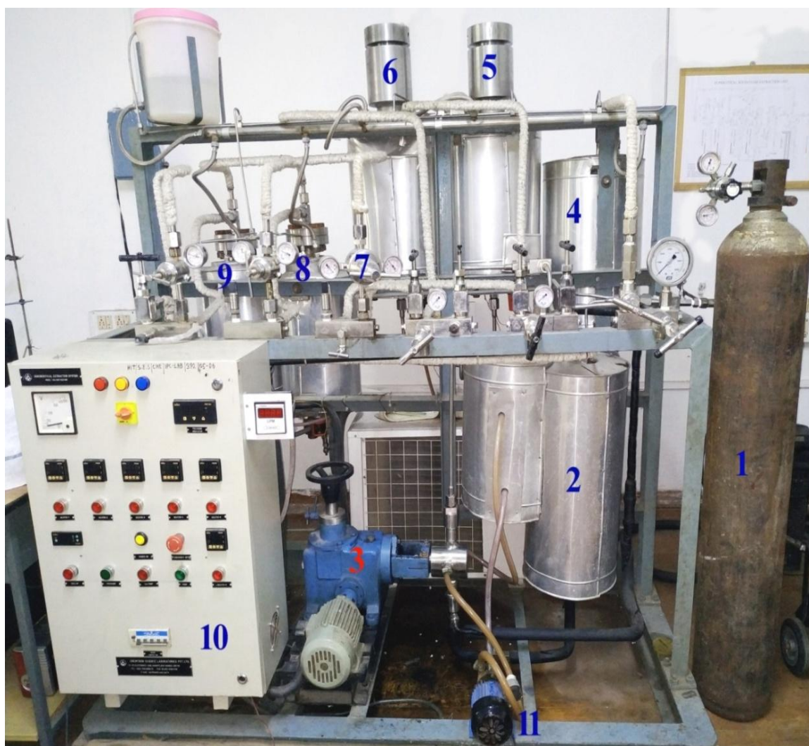
Fig.4.1: Semi-continuous SCO 2 E Experimental Setup (Model No: CSL/SCF/1L2/400)
