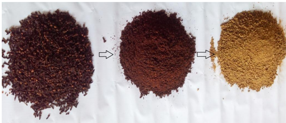
Fig.7.18: Gradual Changes of Colour of Ground Clove Buds before and after SCO 2 E
