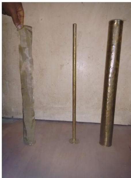
Fig.4.7: Modification of the Cylindrical Feed Shell for Fine Size Particles
