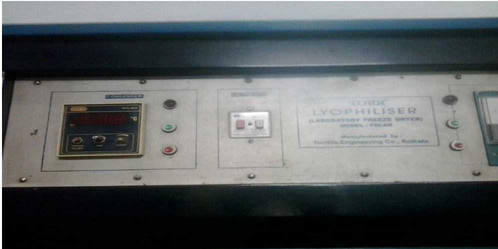
Figure 1.9: Temperature and Vacuum gauge control panel.
