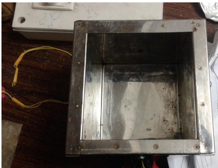
Figure 4.10: Six-sided cubic heater (SS made).
