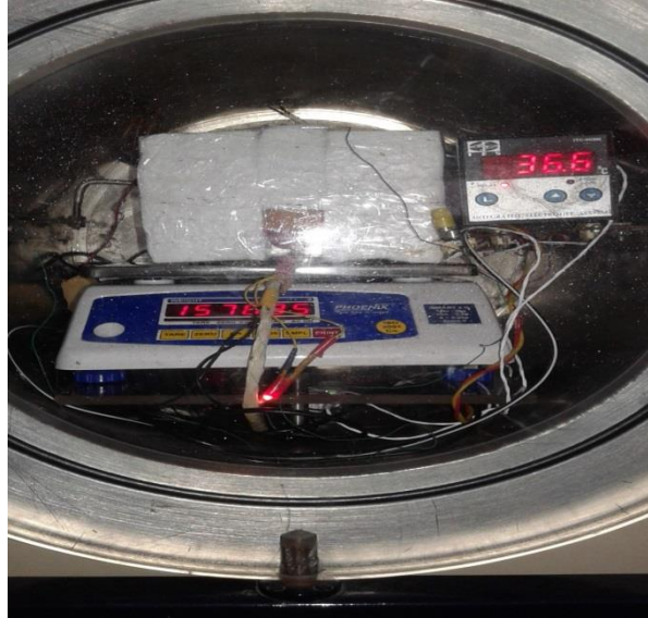
Figure 4.18: Cubic heater (insulated) connected with PID controller: heater rested on weighing balance and placed inside the VD chamber.
