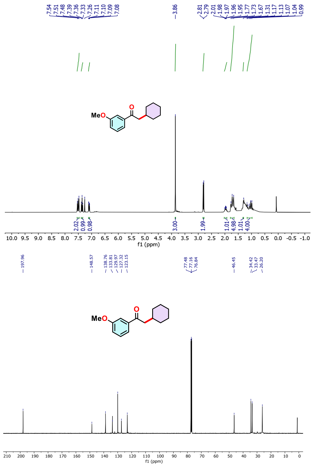
Figure 4.7. 1 H NMR (300 MHz) and 13 C NMR (75 MHz) spectra of compound 3e in CDCl 3 .
