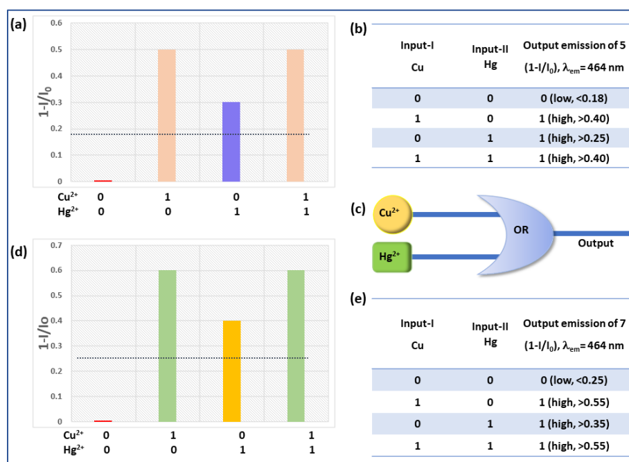
Figure 5.8 (a) Bar diagram, (b) truth table for probe 5 , (c) circuit of the OR logic gate, (d) bar diagram, (e) truth table for probe 7 , taking the fluorescence response for \text{Cu}^{2+} and \text{Hg}^{2+} at 464 nm as the two inputs.
