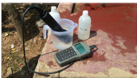
Fig. 2.6 Measurement of physical parameters, using Portable multi parameter system.
