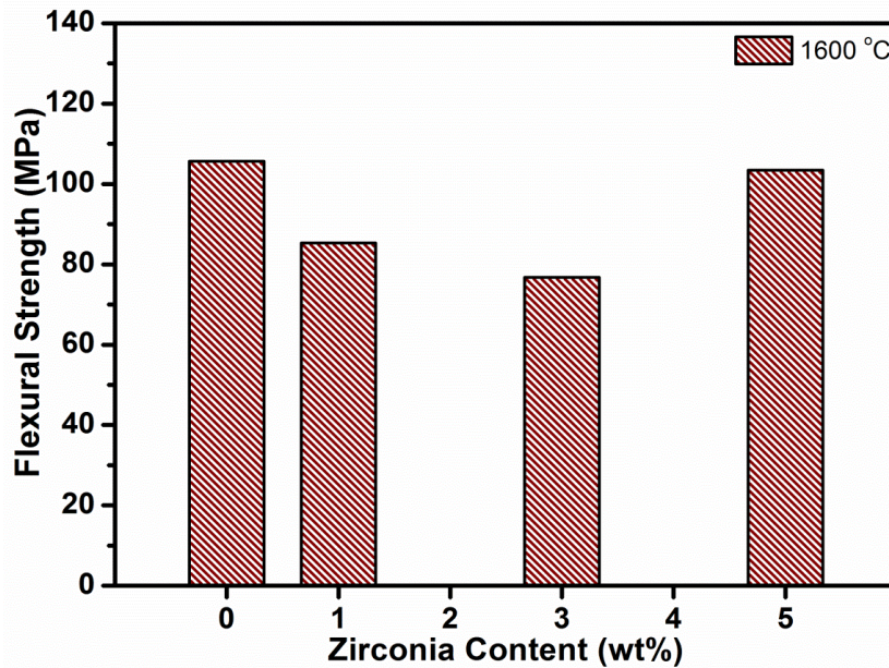
Figure 5-36: Variation in flexural strength at room temperature with zirconia content of the samples sintered at 1600 °C
