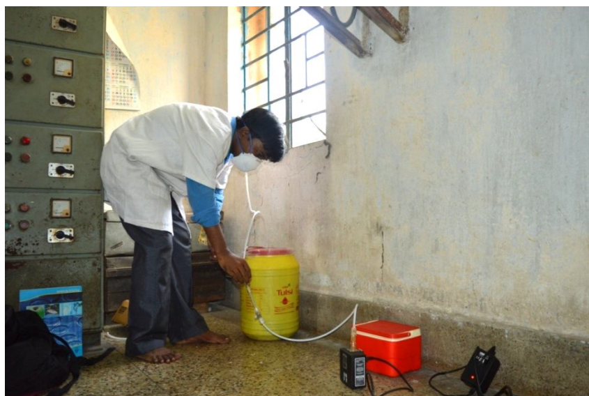
Figure 4.4 Sampling of VOCs from headspace of the jar using an Escort Elf air sampling pump using sorbent tubes.
