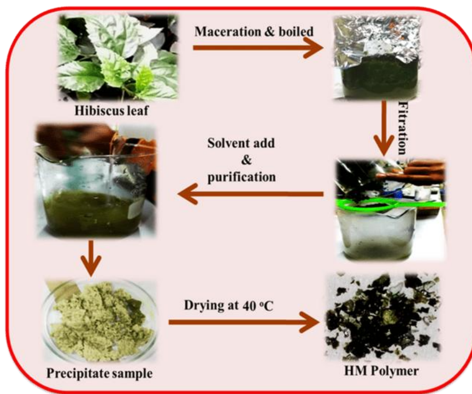
Figure4.1. Diagram represent the fabrication process of Hibiscus mucilage polymer
