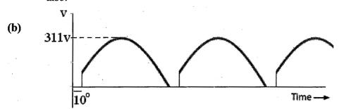
The voltage waveform from a SCR based dimming circuit is shown. What will be the power consumption of a 220V, 40W lamp (resistive) connected to this voltage? To reduce the power consumption by 20% what should be the triggering angle?
