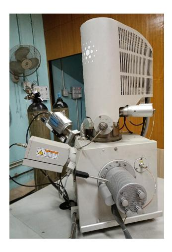
Figure 1.16: Digital image of FESEM instrument.
