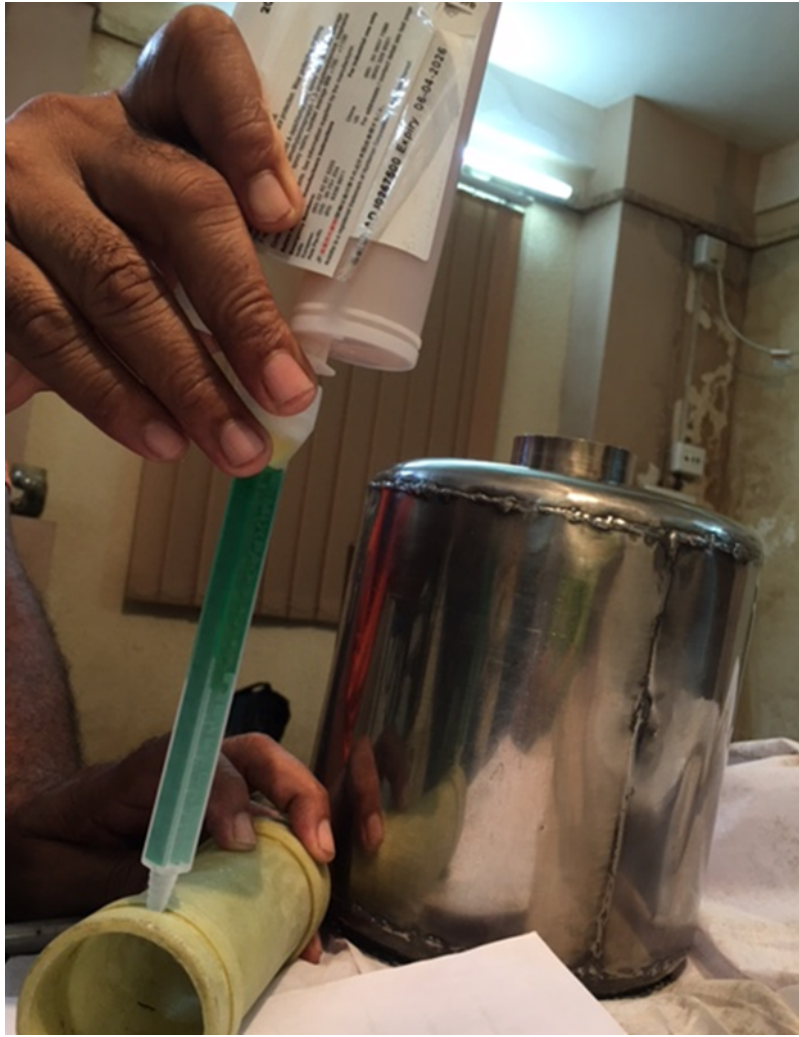
Figure 6F. 4 : Fabrication of FRP Neck with inner vessel with Eco-bond (Epoxy Resin)
