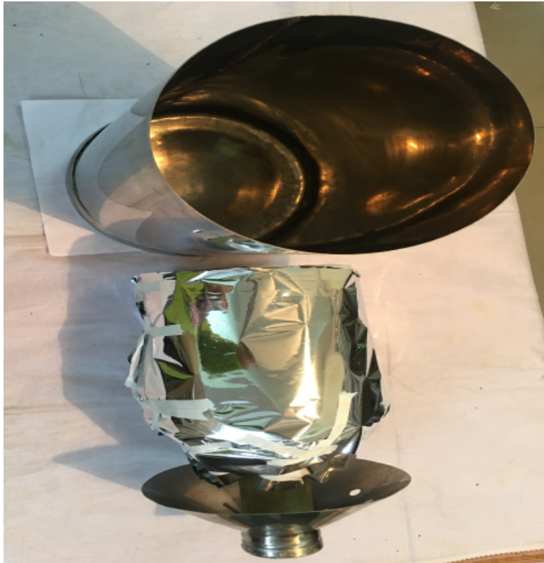
Figure 6F.3 : Pictorial view of the inner stainless steel vessel and outer vessel before assembling
