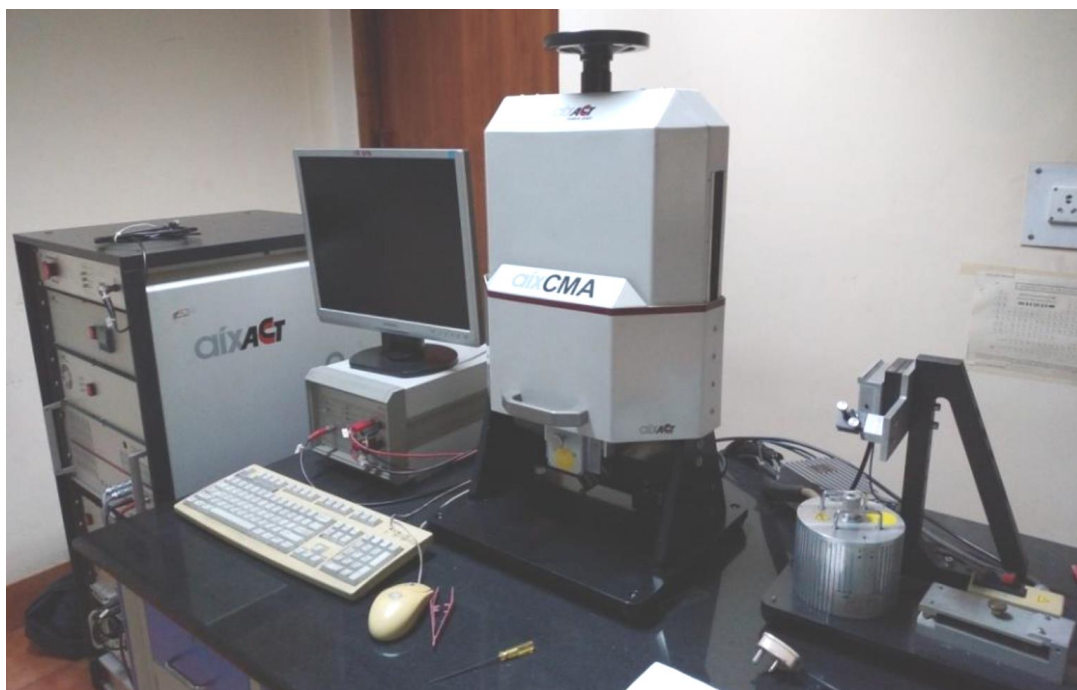
Fig. 2.20 Digital image of the Ceramic Multilayer Actuator Test Bench (aixACCT System GmbH, Germany).
