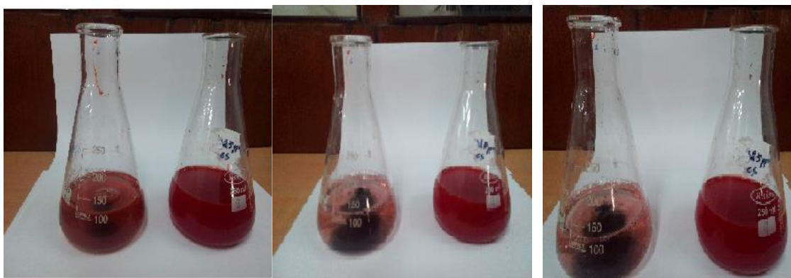
Figure 5.16 CR remove by R-GO Figure 5.17 CR remove by GO Figure 5.18 CR remove by GONC
