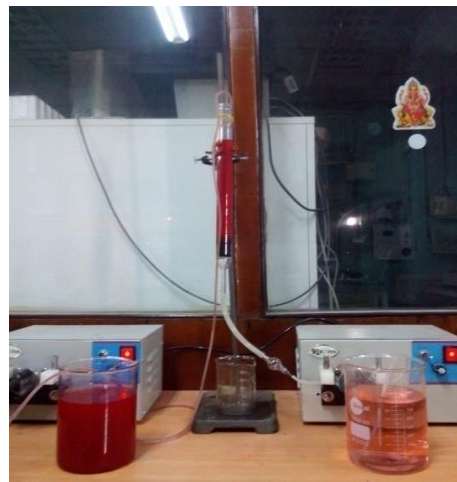
Figure no 5.30 Column study (experimental set-up)
