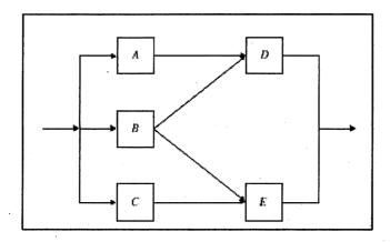
(e) Consider the system shown below. Use the tie-set and cut-set methods to estimate the system reliability.
