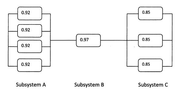
In subsystem A two components must operate for the subsystem to function successfully. Subsystem C has true parallel reliability. Calculate the reliability of each subsystem and overall system reliability. (10)
