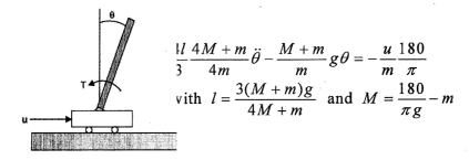
where m is the mass of the pole assumed to be concentrated at the center of the pendulum
