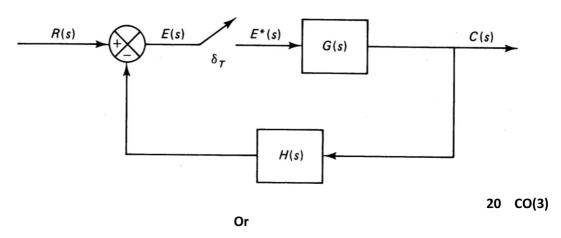
In the Figure above consider that the discrete equivalent of G(s) i.e.  $G(z) = \frac{10z+5}{(z-1)(z-0.2)}$  and H(s)=1.Derive the closed-loop transfer function  $\frac{C(z)}{R(z)}$  and express it in the form of a difference equation.
