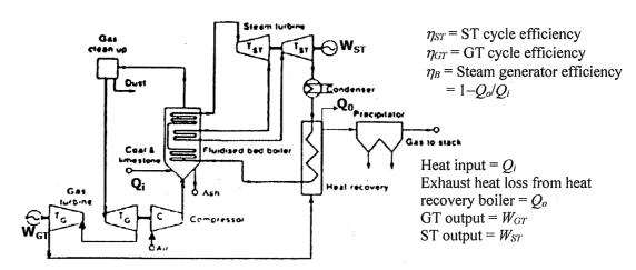
The above figure shows a GTCC combined cycle with a PFBC boiler. Assuming that a fraction x of the supplied heat is received by the gas turbine cycle, calculate the combined cycle efficiency in terms of  $\eta_{ST}$ ,  $\eta_{GT}x$  and  $\eta_{B}$ . 10 marks
