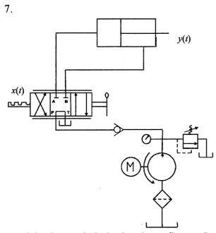
Explain the symbols in the above figure. Consider an actuating mass m and an appropriate form of cylinder friction to obtain the differential equation relating x(t) & y(t) during piston extension assuming oil as incompressible. [20]
