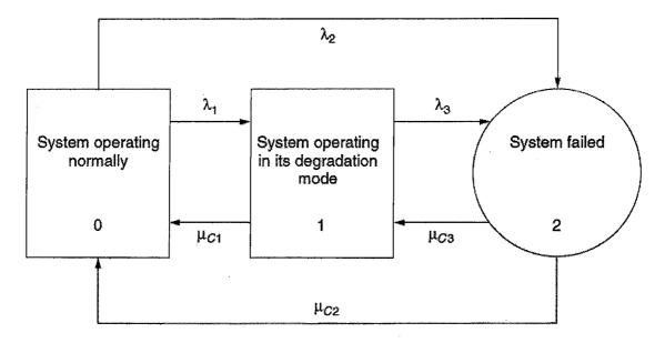
Assume,  $\lambda_1 = 0.002$  failures per hour,  $\lambda_2 = 0.003$  failures per hour,  $\lambda_3 = 0.001$  failures per hour,  $\mu_{c1} = 0.006$  repairs per hour,  $\mu_{c2} = 0.004$  repairs per hour, and  $\mu_{c3} = 0.008$  repairs per hour. Calculate the value of the system full steady-state availability. [4+4+4+8]
