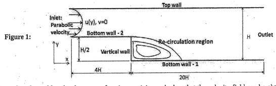
Formulate the problem by the *stream function-vorticity* method so that the velocity field can be obtained. Assume the expression of the inlet parabolic velocity profile as:  $u(y) = \frac{2y}{H} \left( 1 - \frac{2y}{H} \right)$ . (i) Write governing equations along with the boundary conditions. (ii) Formulate with the stream function-vorticity method. (iii) Discretize the
