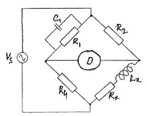
obtained with C1 = 1 nF, R1 = 2.2 M $\Omega$ , R2 = 22.2 k $\Omega$ , R4 = 10 k $\Omega$ . Find the value of the inductance Lx (in mH) and Rx.
