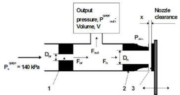
The diameter of the supply restriction 1 is 0.2-0.3 mm (Dor), whereas that of the nozzle (Dn)2 is 0.8 mm . If the distance between the flapper 3 and the nozzle(3) is x, then, show the output gage pressure
