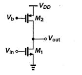
c) What is 1/f corner frequency? In the above circuit, if the width and length are increased by 2x for both the transistors (i.e., keeping aspect ratio unchanged), explain how the corner frequency might change.
