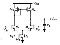
b) Determine the expressions and values of the input common mode range (both ICMR+ and ICMR-) of the above amplifier. Consider  $V_{OV,5} = 100 \text{ mV}$ .
