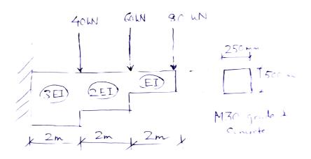
For the beam shown above find the deflection and slope at the free end using Moment-Area Theorem or Conjugate Beam method 5+15
