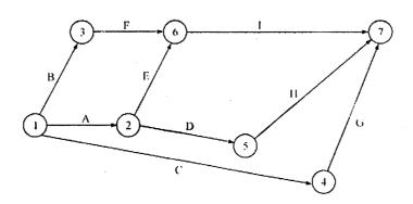
Determine the following: (a) Expected completion time and variance of each activity (b) The earliest and latest expected completion times of each event. (c) The critical path. (d) The probability of expected completion time of the project if the original scheduled time of completing the project is 41.5 weeks. (e) The duration of the project that will have 95 per cent chance of being completed. (For standard normal Z=1.645, area under the standard normal curve from 0 to Z is 0.45)
