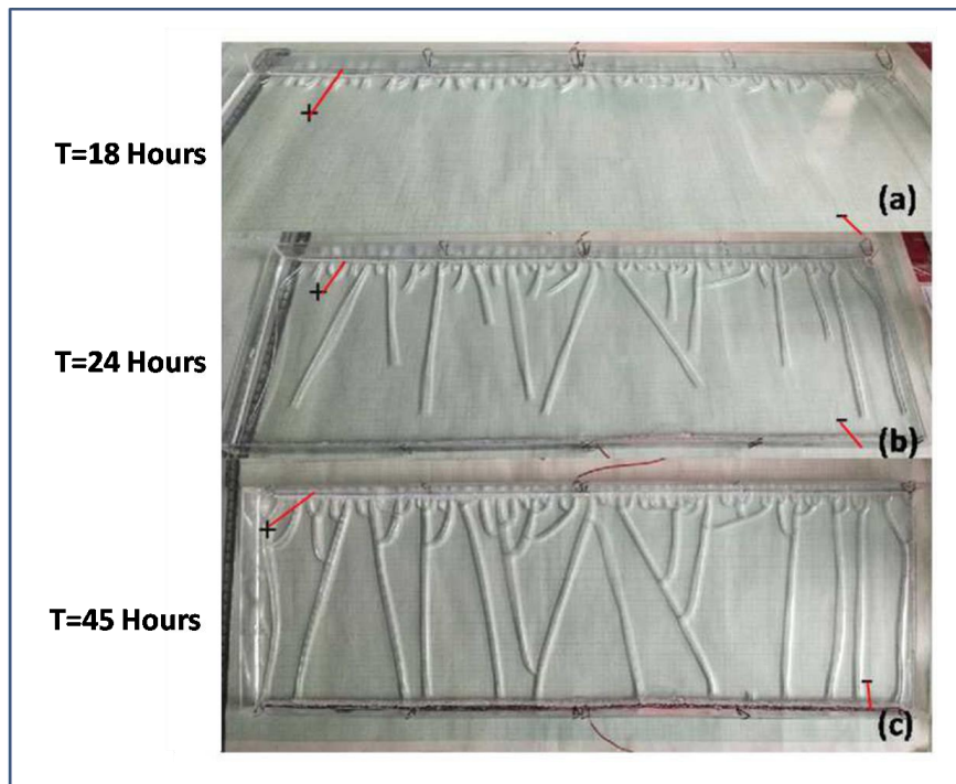
Figure 3.3.(a)–(c) depict the time evolution of the crack patterns created in box 2 at a voltage of 165V. The box is 60 cm in length and 21 cm in width, respectively.
