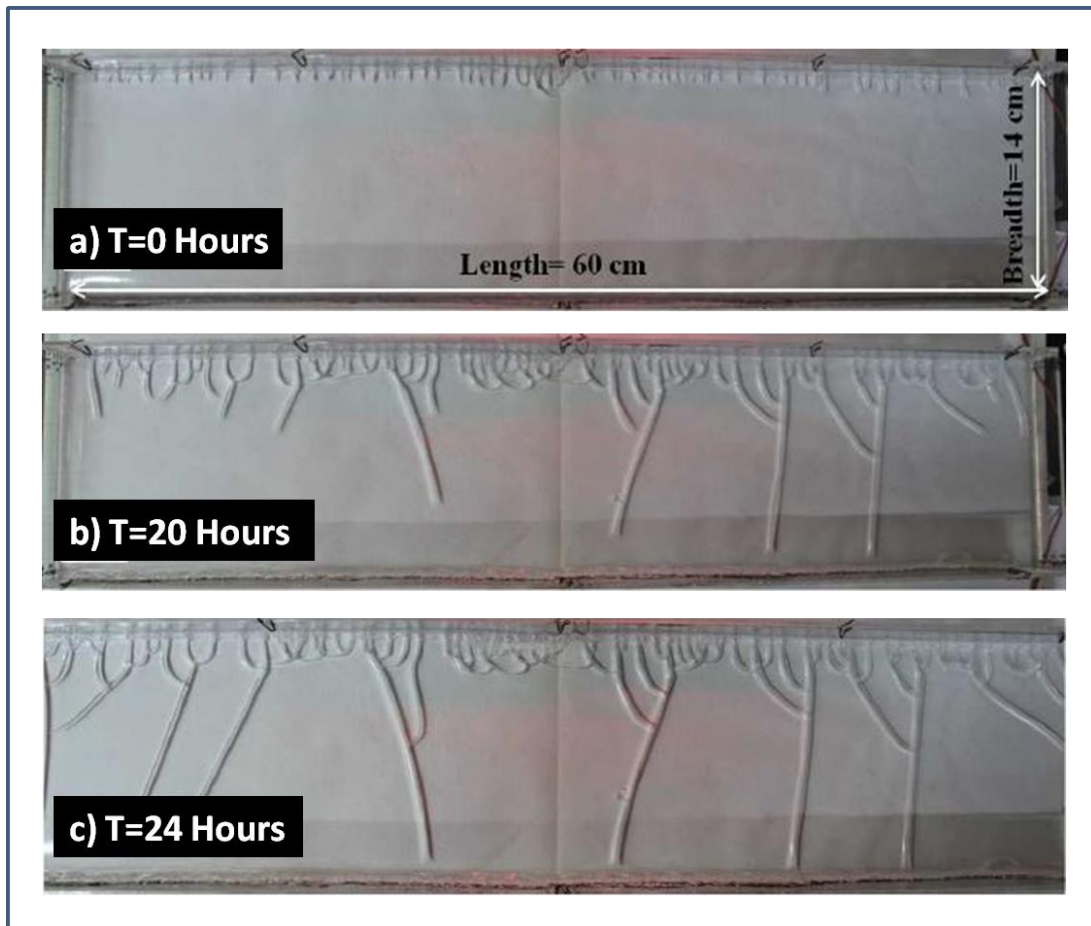
Figure 2.3. (a - c) illustrates how crack patterns developed over time with a voltage of 80 volts.
