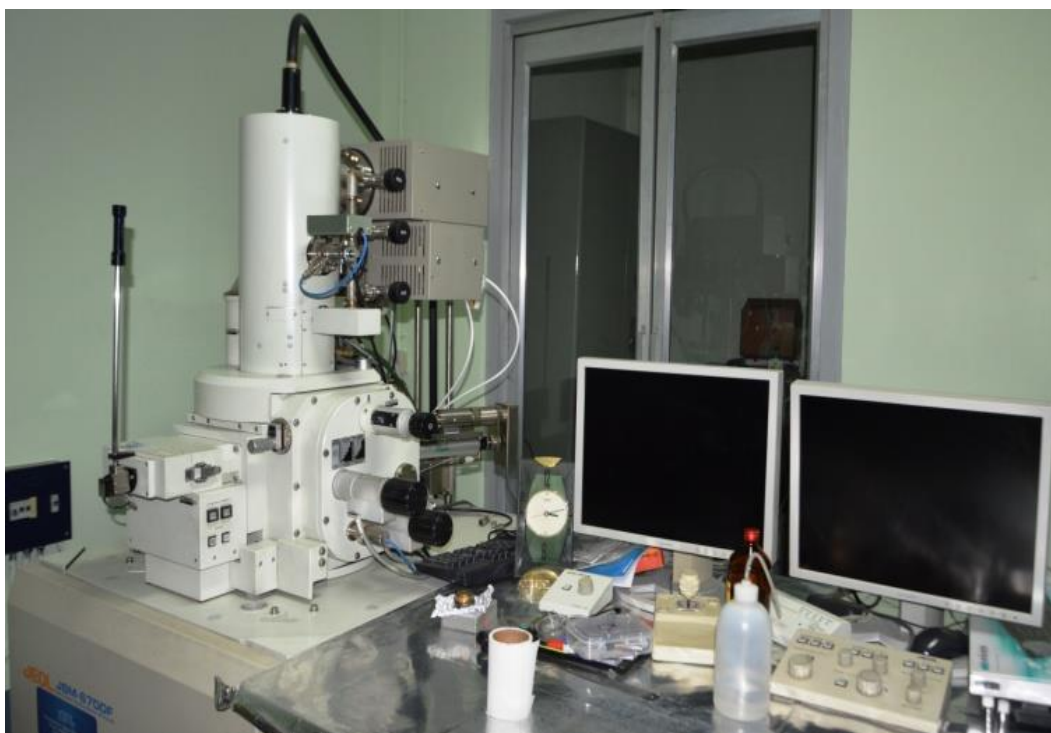
Fig. 3.9: Digital image of FESEM (JEOL, Model: JSM-6700F).
