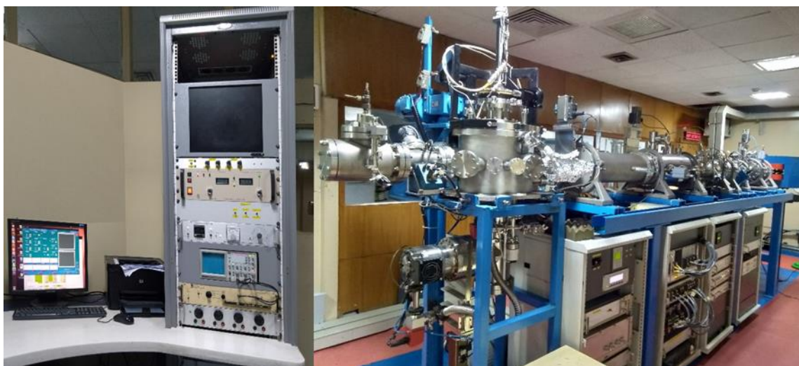
Fig. 3.4: Digital image of the implantation unit of LEIBF at IUAC, New Delhi.
