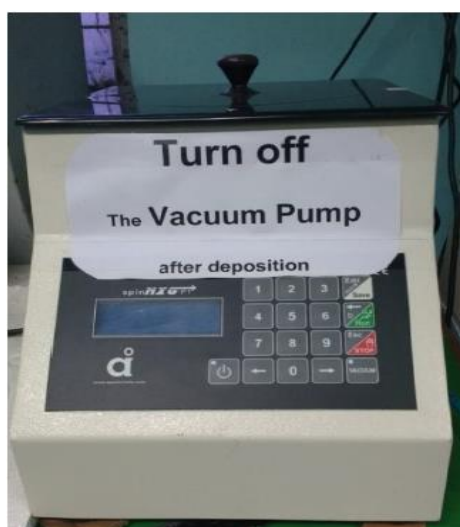
Fig. 3.2: Digital image of the spin coating unit (APEX Instruments, Model: spinNXG-P1) used in the work.
