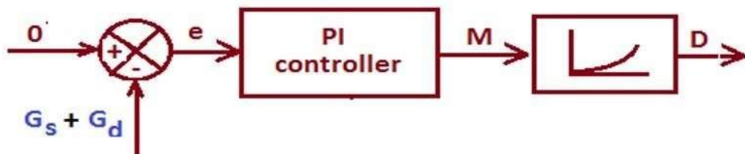
Fig 4.45 Method of implementation for MPPT
