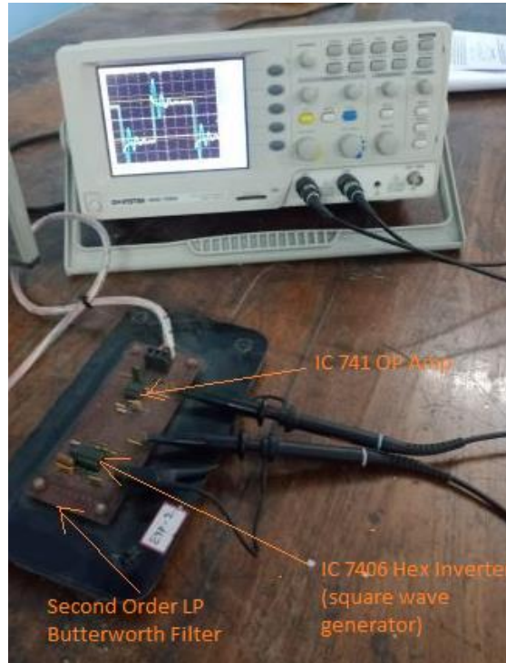
Figure 1 experimental set-up for modelling second-order LP Butterworth filter with an input delay block
