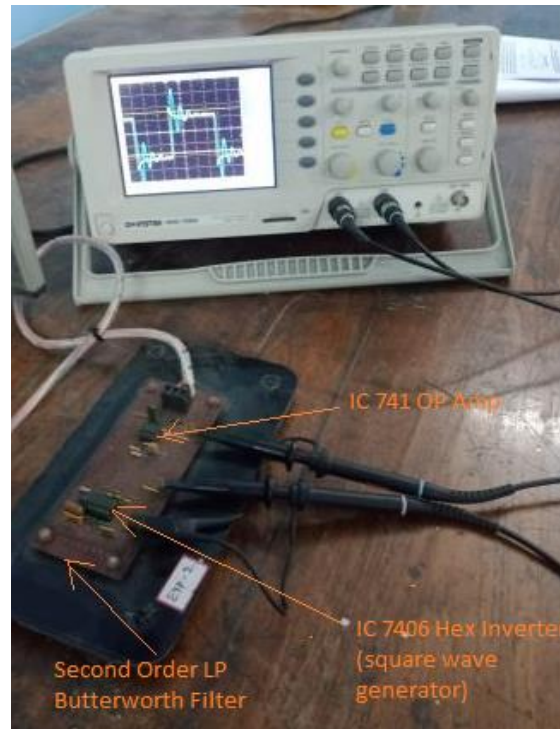
Figure 3.1 Second-order LP Butterworth Filter used in
