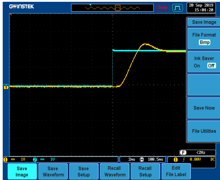
Figure 4.3: Open loop FSM output with an input of 0-2V square wave of freq. 15Hz acquired in DSO
