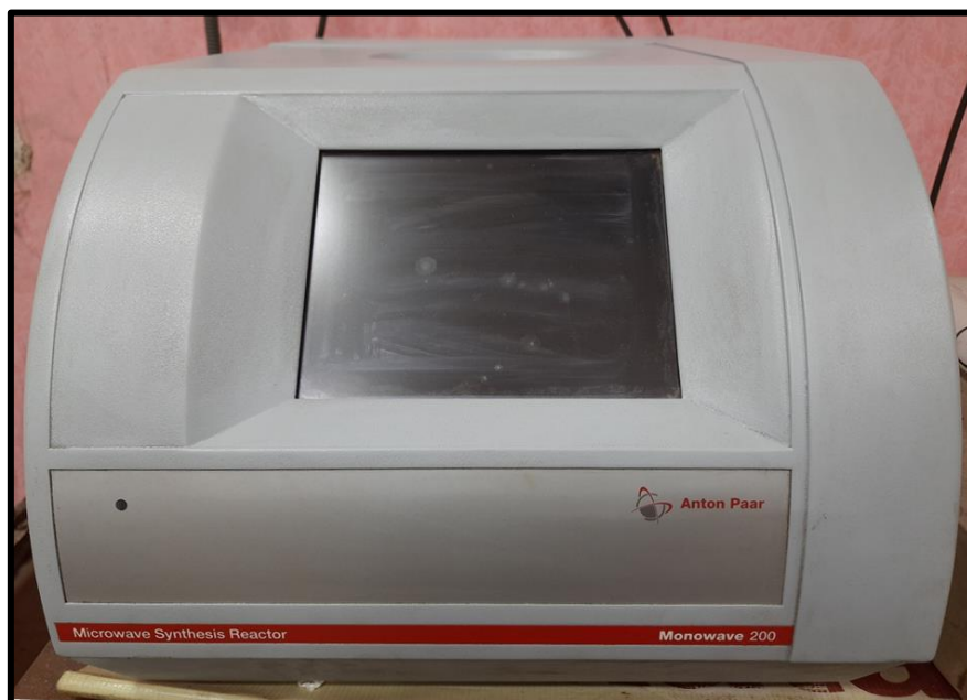
Figure 3.4 Digital photograph of the Monowave 200 microwave synthesis reactor from Anton Paar.
