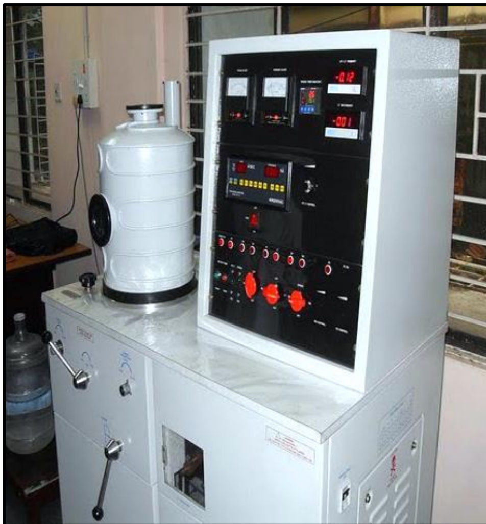
Figure 3.10 Digital photograph of the HIND HIVAC make thermal evaporation-based vacuum coating unit (model: 12A4D).
