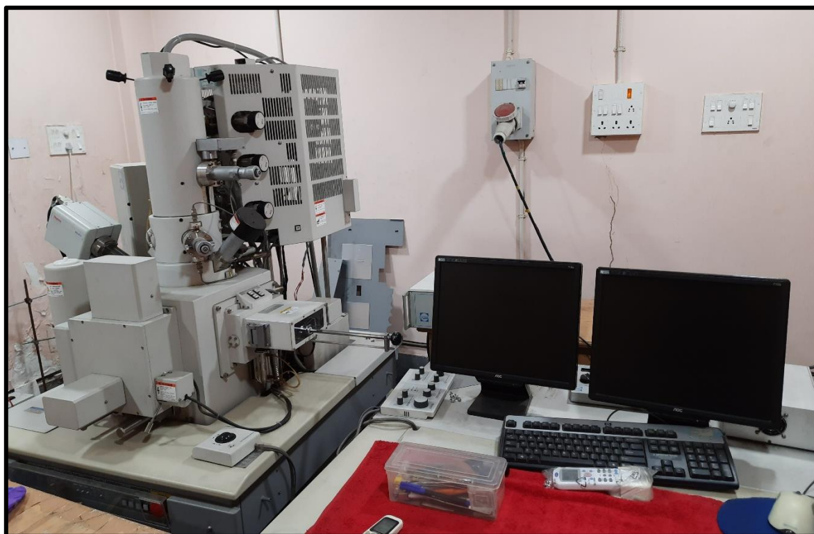
Figure 3.16 Digital photograph of the Hitachi S-4800 FESEM and EDX facility.
