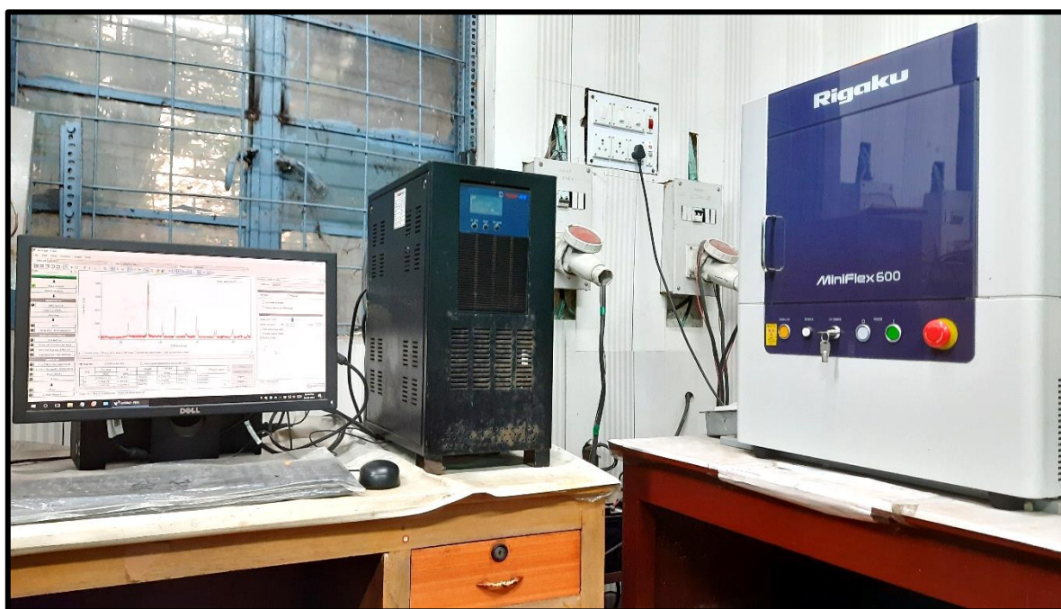
Figure 3.11 Digital photograph of the Rigaku MiniFlex 600 powder X-ray diffractometer.
