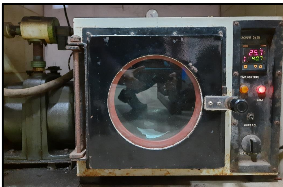
Figure 3.3 Digital photograph of the vacuum oven (maximum temperature: 120 °C).
