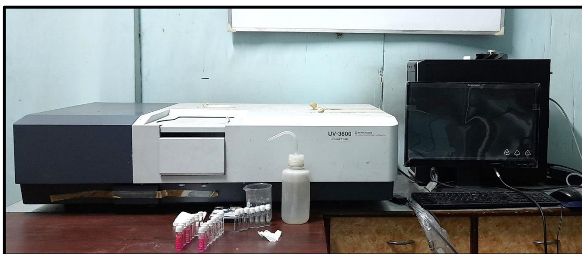
Figure 3.15 Digital photograph of the Shimadzu UV-3600 UV-Vis-NIR spectrophotometer.
