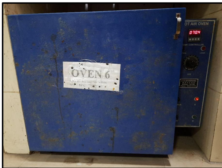
Figure 3.2 Digital photograph of a hot-air oven (maximum temperature: 180 °C).
