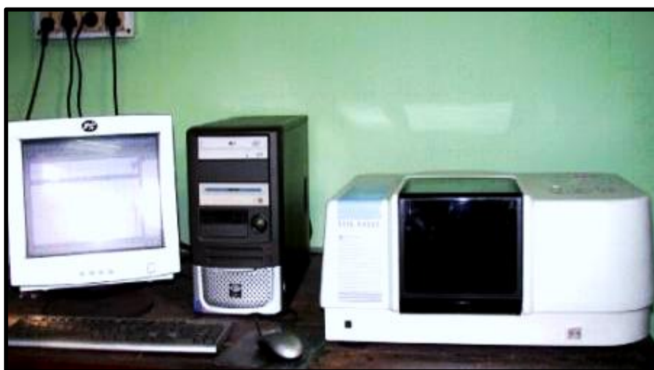
Figure 3.14 Digital photograph of the Shimadzu FTIR-8400S spectrometer.
