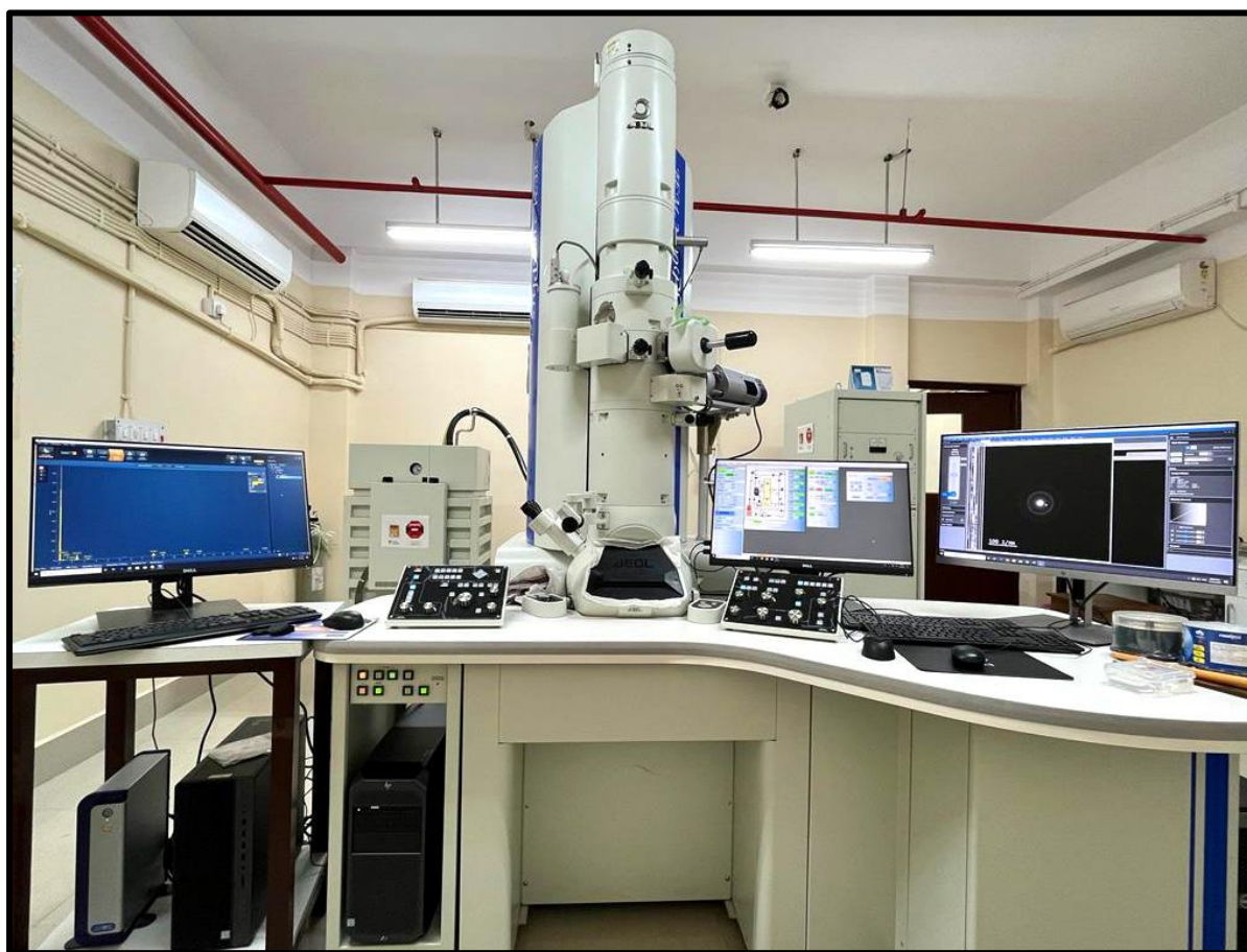
Figure 3.17 Digital photograph of the JEOL-JEM 2100 HRTEM system.
