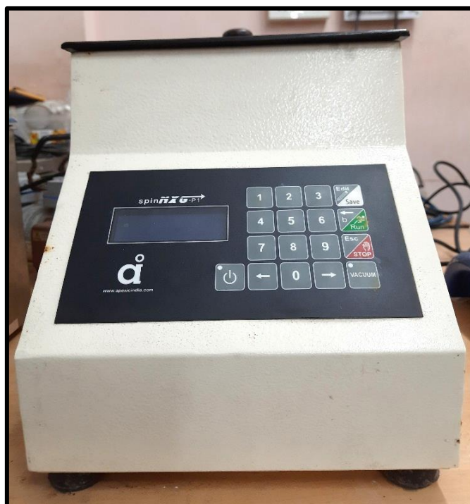
Figure 3.9 Digital photograph of the Apex Spin NXG-P1 spin-coating unit.
