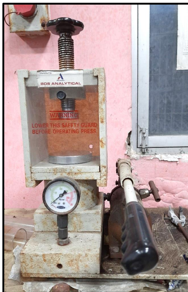
Figure 3.8 Digital photograph of the BDS Analytical standard pelletizer.
