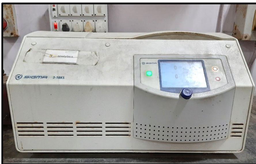
Figure 3.7 Digital photograph of the SIGMA centrifuge machine with built-in cooling facility.
