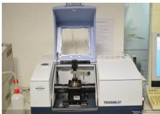
Figure1.12. Photograph of FTIR Instrument and FTIR principle (adopted from webpage, www.google.com )
