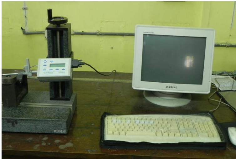
Figure 2.14: Surface Roughness Tester (Surtronic 3+, Taylor Hobson)
