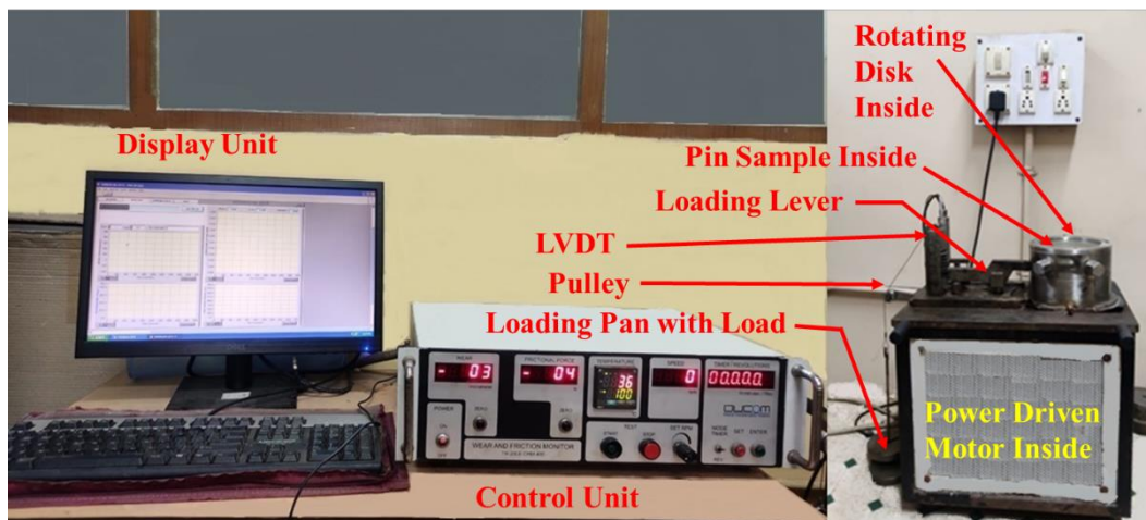
Figure 2.21: Pin-on-disk Tribotester (TR-20LE-CHM-400, DUCOM, India)
