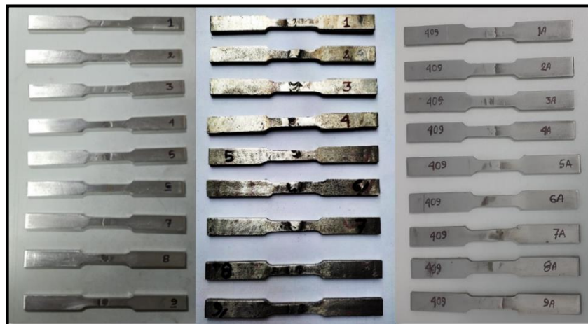
Tensile test samples preparation in milling machine
