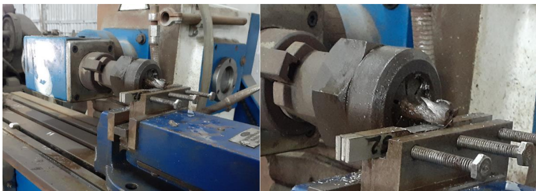
Tensile test samples preparation in milling machine
