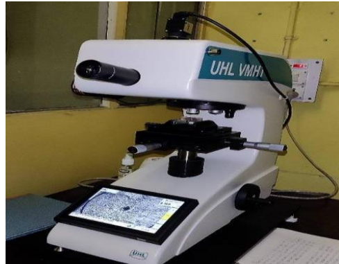
Figure 3.6 Micro hardness testing machine
