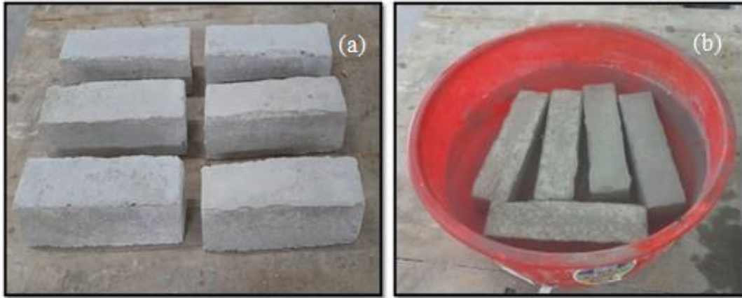
Fig. 4.9: Beam specimens for flexural strength test.
