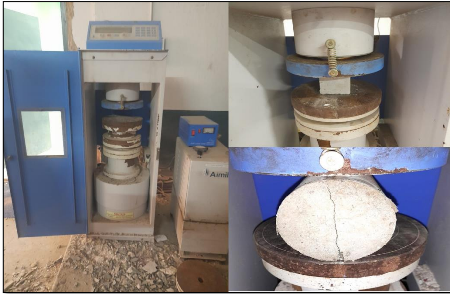
Fig. 3.2: Compressive strength and split tensile strength test set up.
