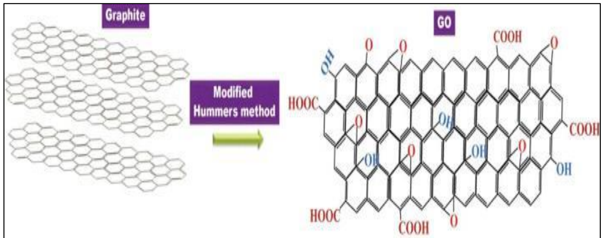
Fig. 1.4: Modified Hummer's method for GO synthesis.
