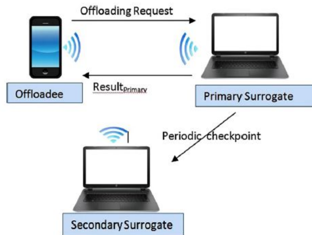
Figure 5.4: Offloading scheme depicting the responsibility of a primary surrogate, S_p and a secondary surrogate, S_s
