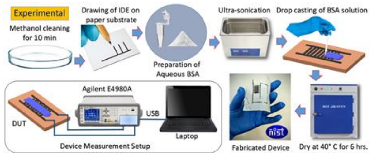
FIG. 4.7. Process of fabricating IDE based device on paper substrate.
