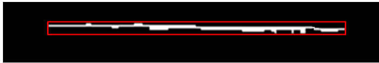
FIGURE 3.4: A sample thresholded u-depth map with a segmented obstacle and the corresponding bounding box.
