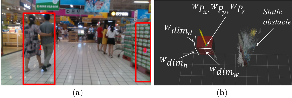
FIGURE 3.9: (a) An RGB snapshot with detected obstacles in the OpenLORIS-Scene market data [58], (b) Corresponding Rviz [99] visualization with annotated dimensions.
