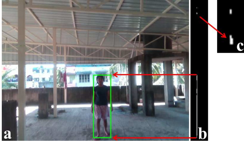
FIGURE 3.7: Estimation of the height of an obstacle using the proposed restricted v-depth map: (a) The same image used in Fig. 3.5 and the result of the proposed technique, (b) Result of the thresholded restricted v-depth map, (c) The magnified view of the thresholded restricted v-depth map shows the portion of the roof as a separate obstacle.
