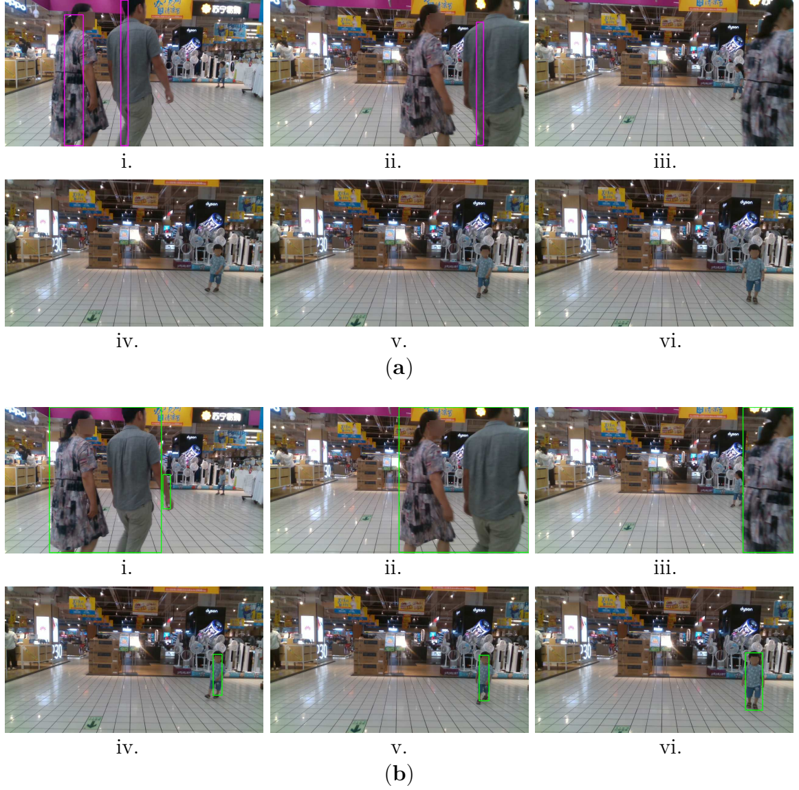
FIGURE 3.22: Comparison of the proposed method with the VbOAD [4] algorithm on the market sequence of the Open LORIS-Scene dataset [58] with multiple dynamic obstacles of different sizes: (a) (i–vi) Time-sampled snapshots with the output of VbOAD, (b) (i–vi) Time-sampled snapshots with the output of our proposed method.
