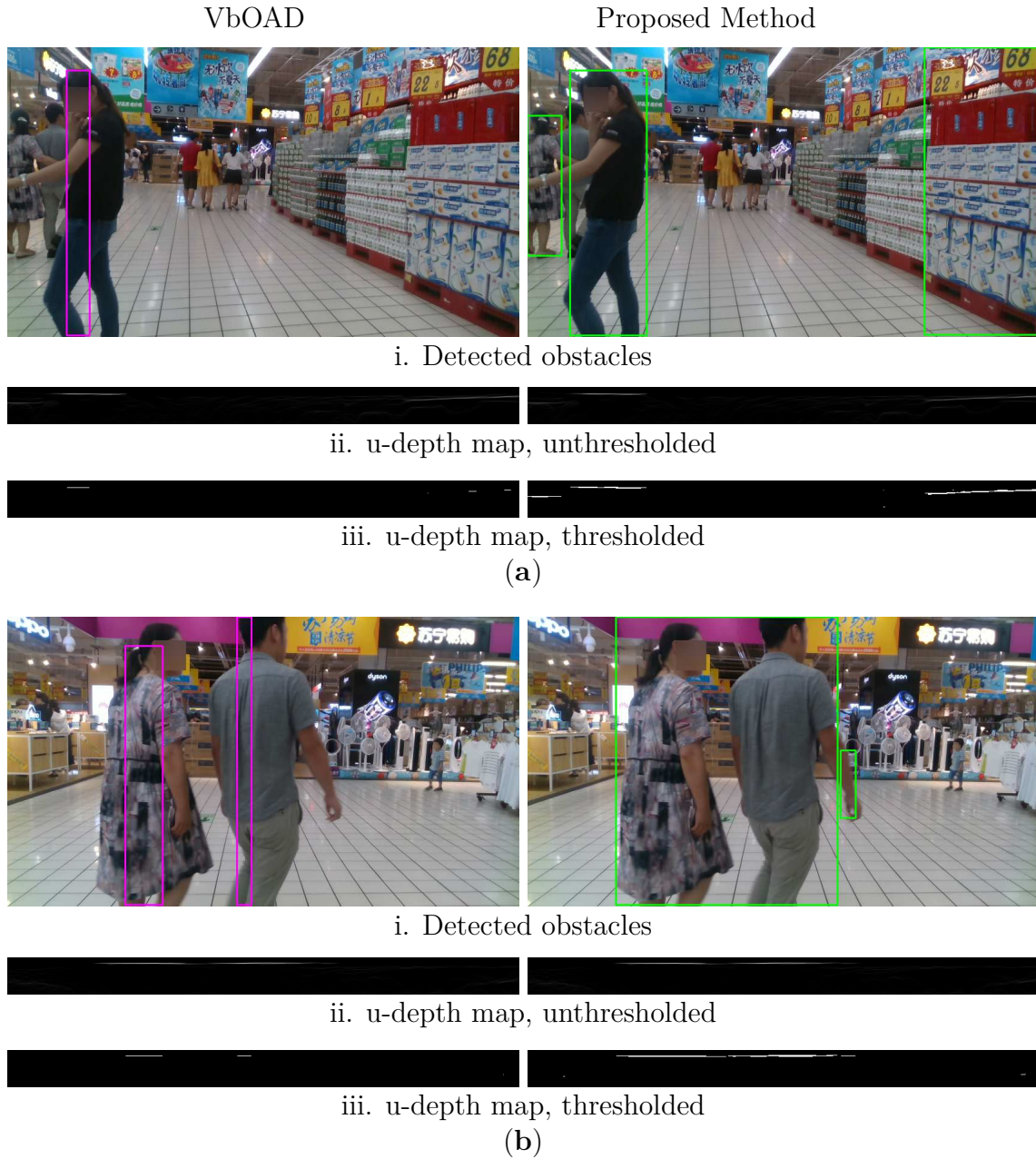
FIGURE 3.23: The effectiveness of the proposed dynamic thresholding compared to fixed thresholding as presented in VbOAD [4] on the market sequence of the Open LORIS-Scene dataset [58]: (a) Example 1, (b) Example 2.
