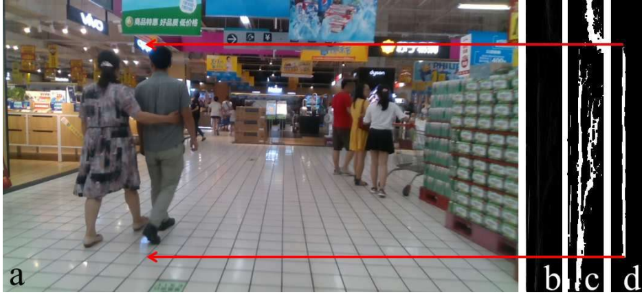
FIGURE 3.6: Obstacle height calculation using the proposed restricted v-depth map: (a) The same snapshot from Fig. 3.3(a), (b) Corresponding v-depth map, (c) Corresponding thresholded v-depth map, (d) Corresponding proposed thresholded restricted v-depth map.
