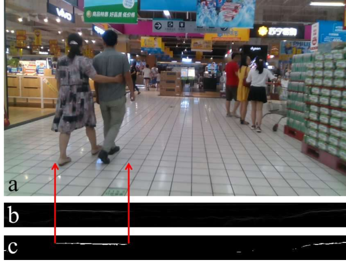
FIGURE 3.3: Estimating obstacle width from u-depth map: (a) Snapshot from the OpenLORIS-Scene market data sequence [58], (b) Corresponding u-depth map, (c) Corresponding thresholded u-depth map after a closing operation.
