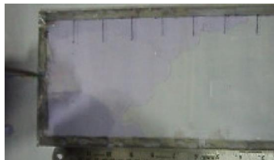
Fig.: Flow Pattern of Water for 0.7 mm thin Rectangular Plate in Flat Position
