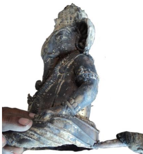
(e) Unfinished Cast Model with Side Gating System
