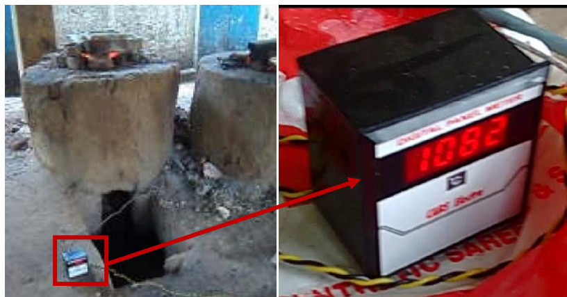
Figure-4.8: K-Type Thermocouple with Digital indicator: The steel probe of the thermocouple put in the crucible at the Furnace to measure the temperature
