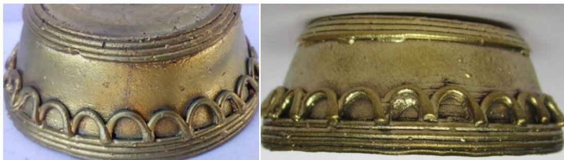
(a) Surface of Cosmetics Case of Type-I Gating System of two Opposite Surface
