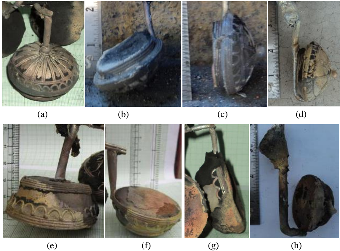
Figure- 7.12: Pictorial View of casting with gating system. Cosmetics Cap (a) Type-I, (b) Type-II, (c) Type-III, (d) Type-IV and Cosmetics Case (e) Type-I, (f) Type-II, (g) Type-III, (h) Type-IV
