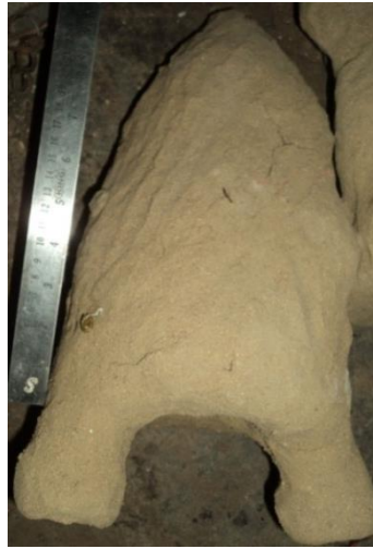
(b) Clay Mold with Top Gating System
