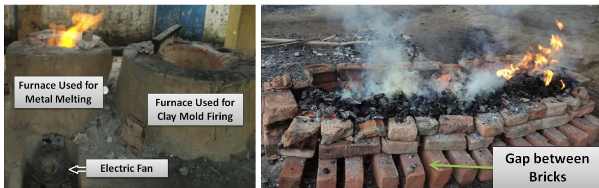
Figure: Permanent Furnace at Bikna (left), Temporary Furnace at Guskara, (Right)
