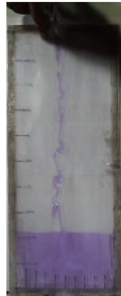
Fig.: Flow Pattern of Water for 0.7 mm thin Rectangular Plate in Vertical Position
