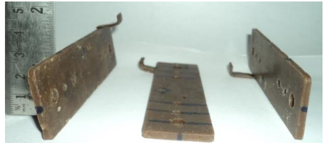
(g) Three gating hystem of solid plate
