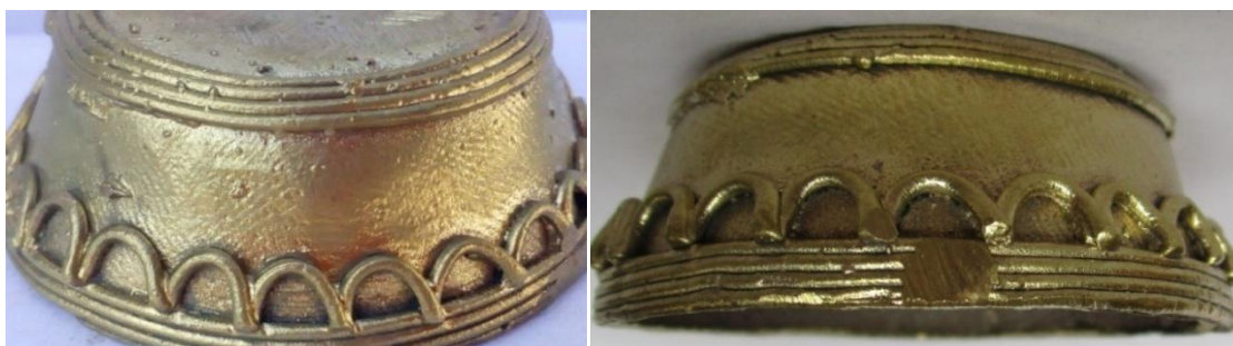
(b) Surface of Cosmetics Case of Type-II Gating System of two Opposite Surface
