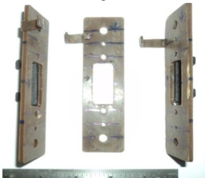
(h) Three gating system of cored plate
