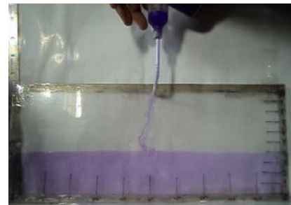
Fig.: Flow Pattern of Water for 0.7 mm thin Rectangular Plate in Horizontal Position
