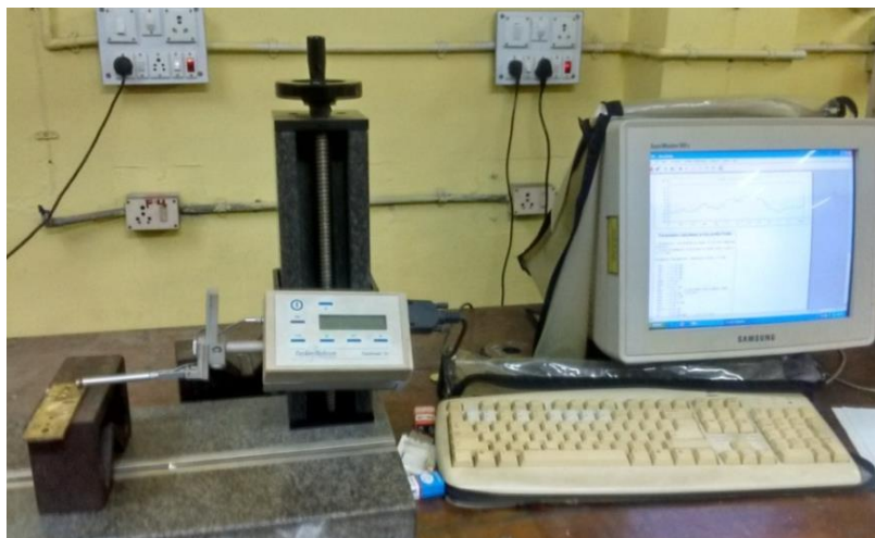
Figure-4.3: Surface Roughness Measuring Machine: Taylor-Hobson instrument
