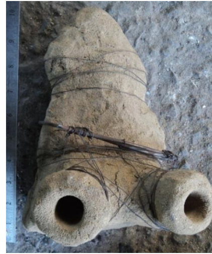
(c) Clay Mold with Side Gating System
