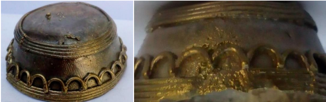
(d) Surface of Cosmetics Case of Type-IV Gating System of Two Opposite Surface
