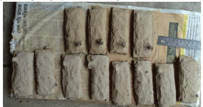
(i) Clay mold of all plates with gating
