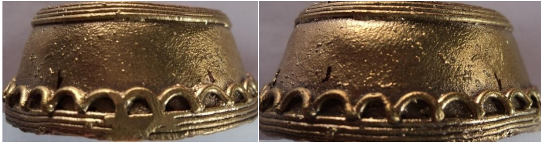
(c) Surface of Cosmetics Case of Type-III Gating System of two Opposite Surface
