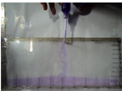
Fig.: Flow Pattern of Water for 0.7 mm thin Rectangular Plate in Horizontal Position
